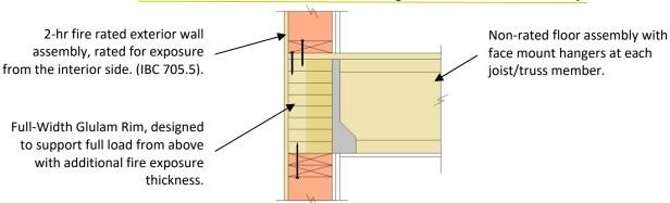
Detail B: 2-hr Exterior Wall Intersecting Non-Rated Floor Assembly
