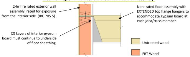
Detail C: Typical 2-hr Exterior Balloon Framed Wall Assembly
